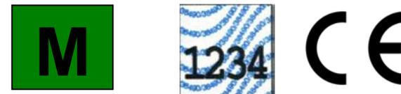
Note the number shown can be different. Measuring equipment, such as length measures or beer glasses may be marked with the CE mark, the M mark and number.
